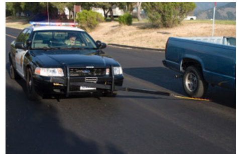
The MobileSpike device enables officers to stop pursuits from the safety of their vehicle with a push of a button (photo provided by MobileSpike).
