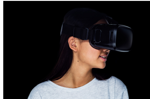
Figure 18: The Tobii VR4 Eye Tracking Platform leverages the HP Reverb G2 Omniconcept Edition to enable detection of eye movements and measurements of pupil dilation (pupillometry), which can be used together with input from a photoplethysmography sensor for measuring heart rate. (Image provided by Tobii)
